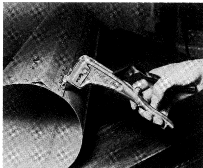
Insert Rivet in predrilled hole and squeeze Handles until mandrel breaks.
