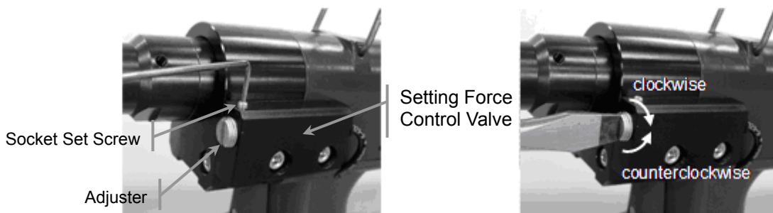
Figure 14: Adjustment of Setting Force
